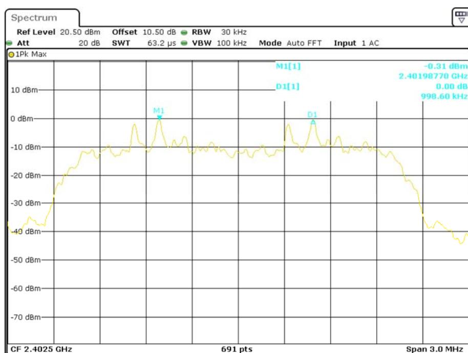
**EDR ( $\pi/4$ -DQPSK): Middle Channel**
