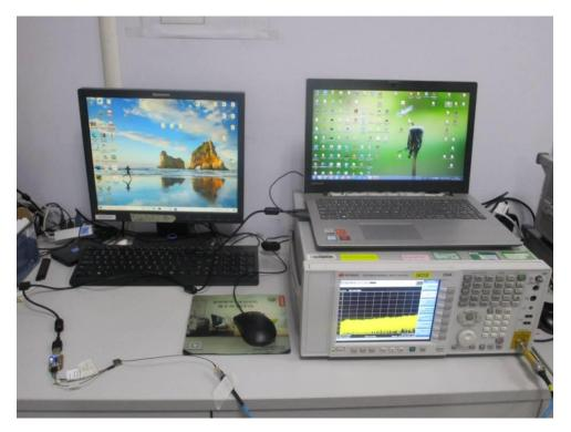
Conducted Emissions at Mains Terminals (150kHz-30MHz)
