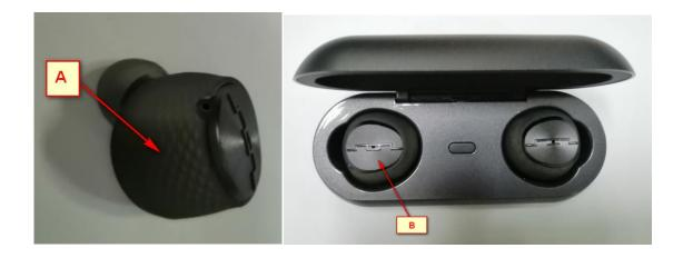
Conclusion: Based on the above description of area A to B, we conclude that the device is unquestionably too small for enabling the FCC ID to be printed onto any surface. We therefore request to move the FCC ID to the user manual and charging case.
