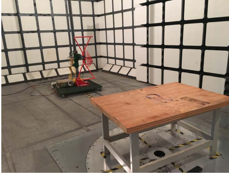
Radiated Emissions View (Below 1 GHz)
