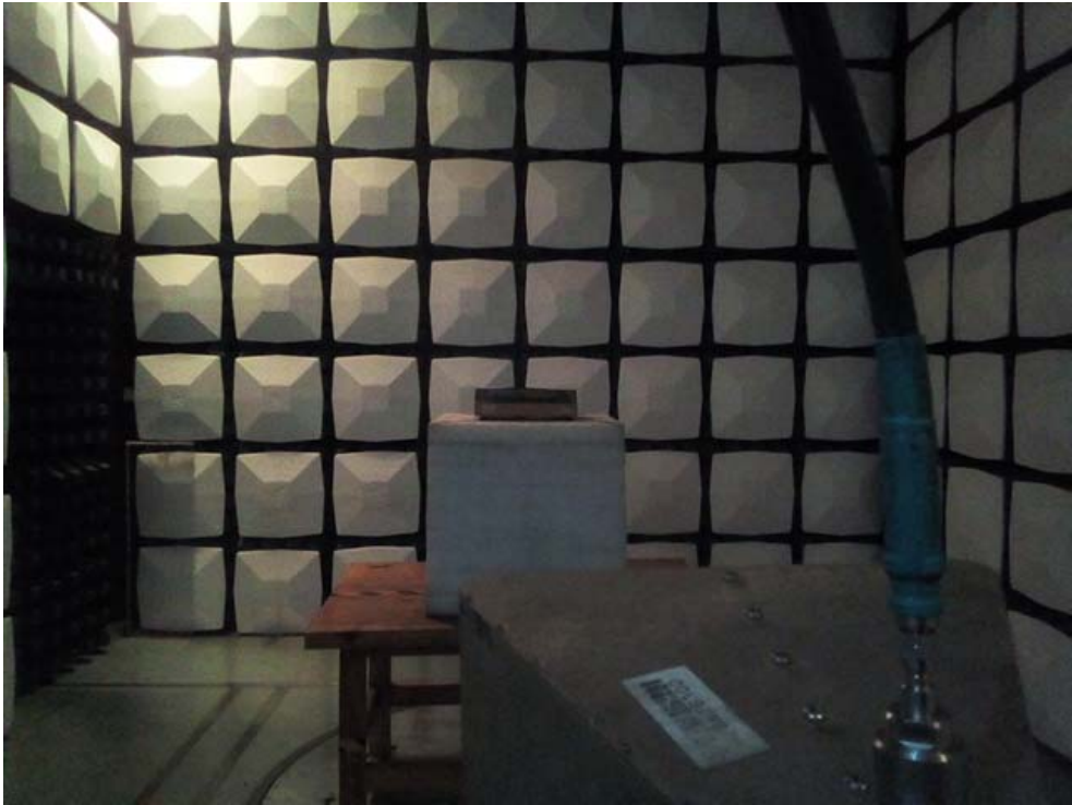
Radiated Emission Above 1GHz View
