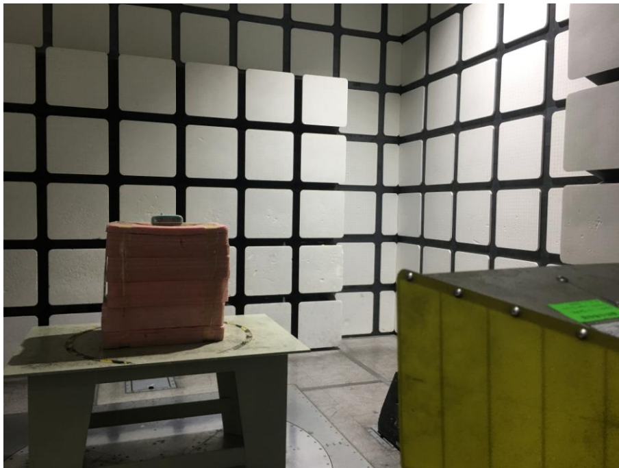
Radiated Emissions View (Above 1 GHz)
