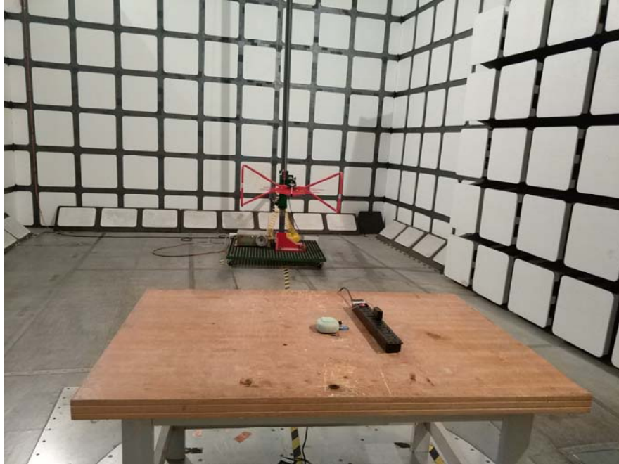
Radiated Emissions View (Below 1 GHz)
