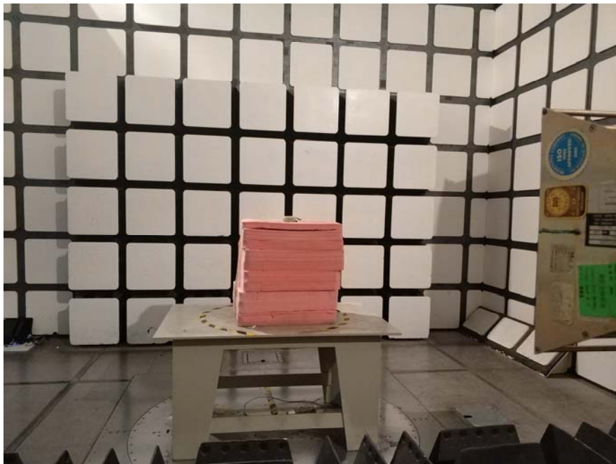
Radiated Emissions View (Above 1 GHz)
