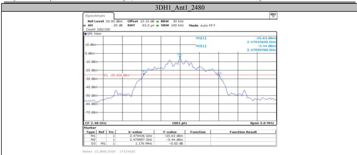
**Appendix B: Occupied Channel Bandwidth****Test Result**
