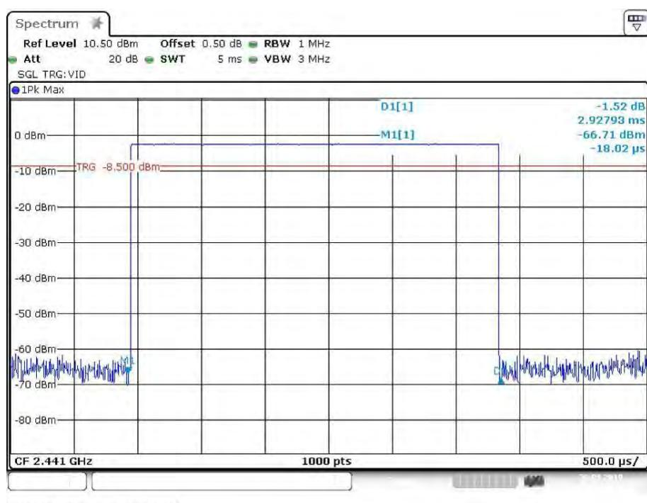
**Pulse time, High Channel, DH5**
