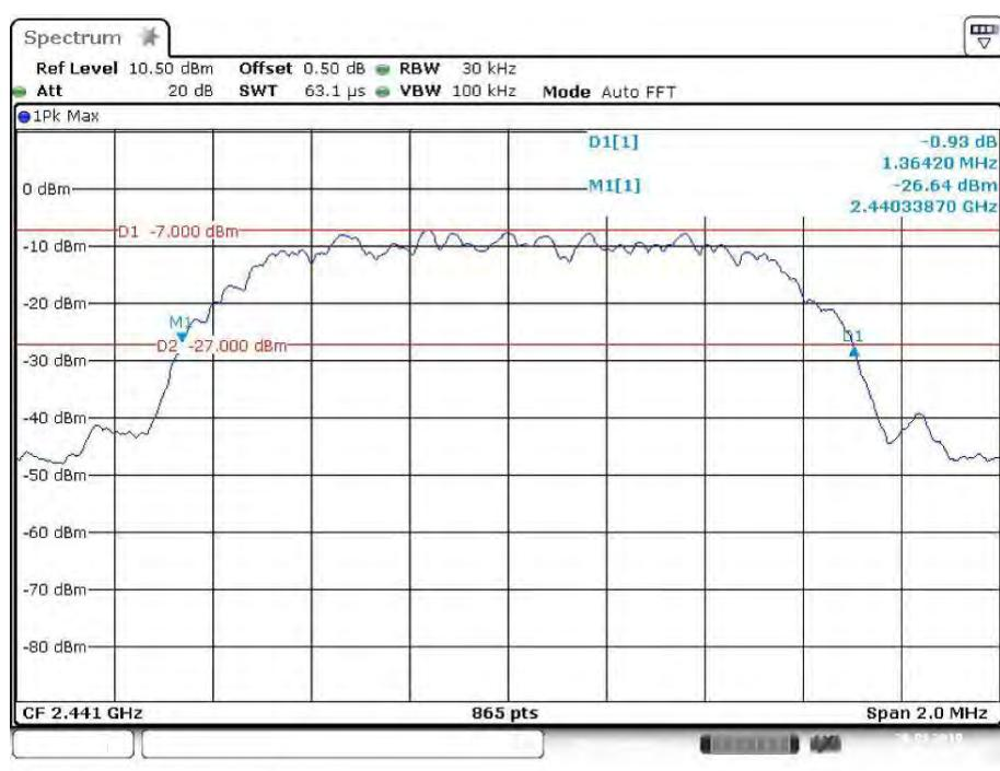
**EDR ( $\pi/4$ -DQPSK): High Channel**
