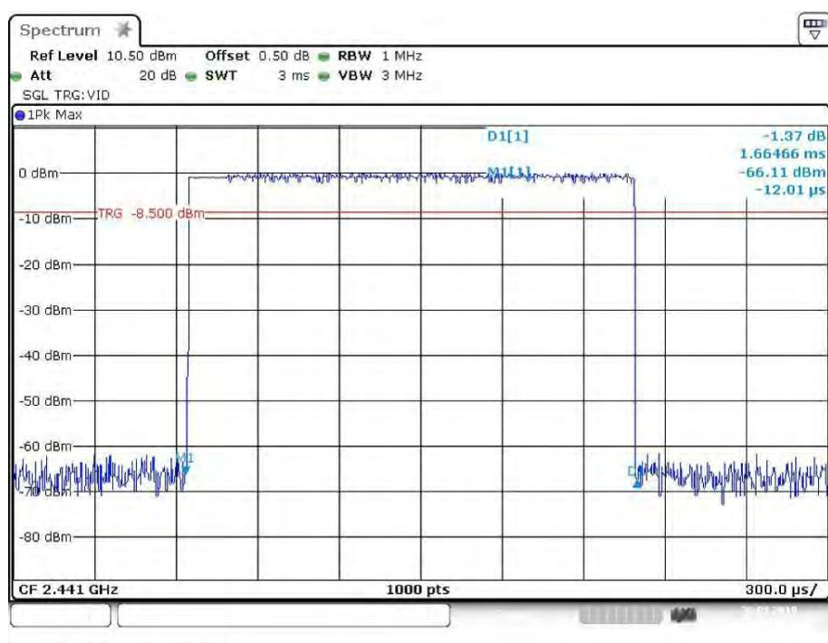
**Pulse time, High Channel, 2DH3**
