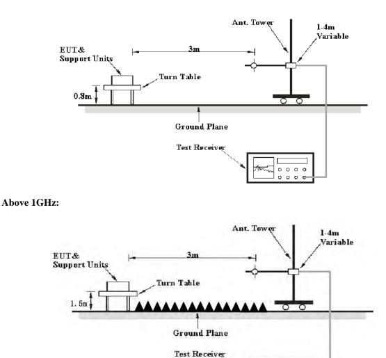
The radiated emission tests were performed in the 3 meters, using the setup accordance with the ANSI C63.10-2013. The specification used was the FCC 15.209 and FCC 15.247 limits.
