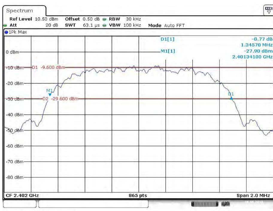
**EDR (8DPSK): Middle Channel**
