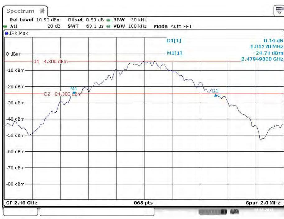
**EDR ( $\pi/4$ -DQPSK): Low Channel**
