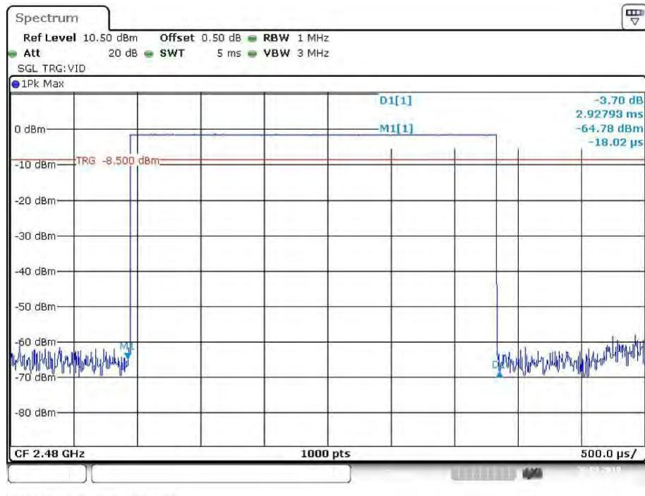
**EDR ( $\pi/4$ -DQPSK):****Pulse time, Low Channel, 2DH1**
