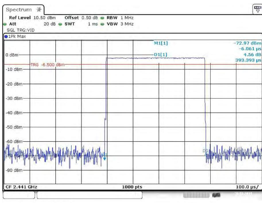
**Pulse time, High Channel, DH1**
