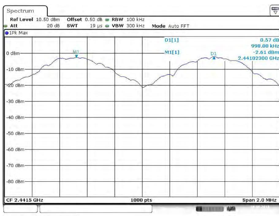
**BDR (GFSK): High Channel**
