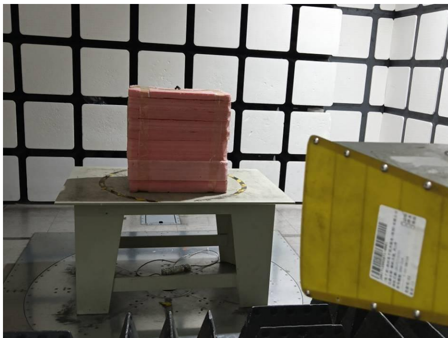
Radiated Emissions View (Above 1 GHz)
