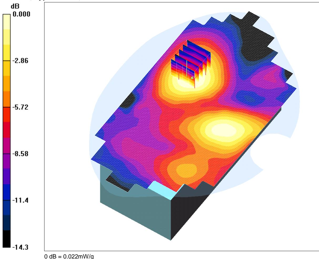
Communication System: EGPRS 1900; Frequency: 1879.8 MHz; Duty Cycle: 1:4
