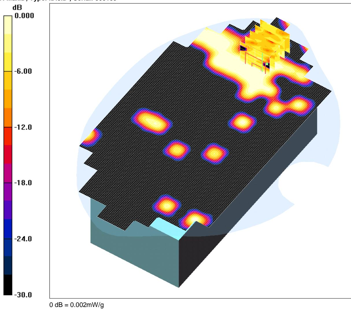
Communication System: WLAN; Frequency: 2437 MHz; Duty Cycle: 1:1
