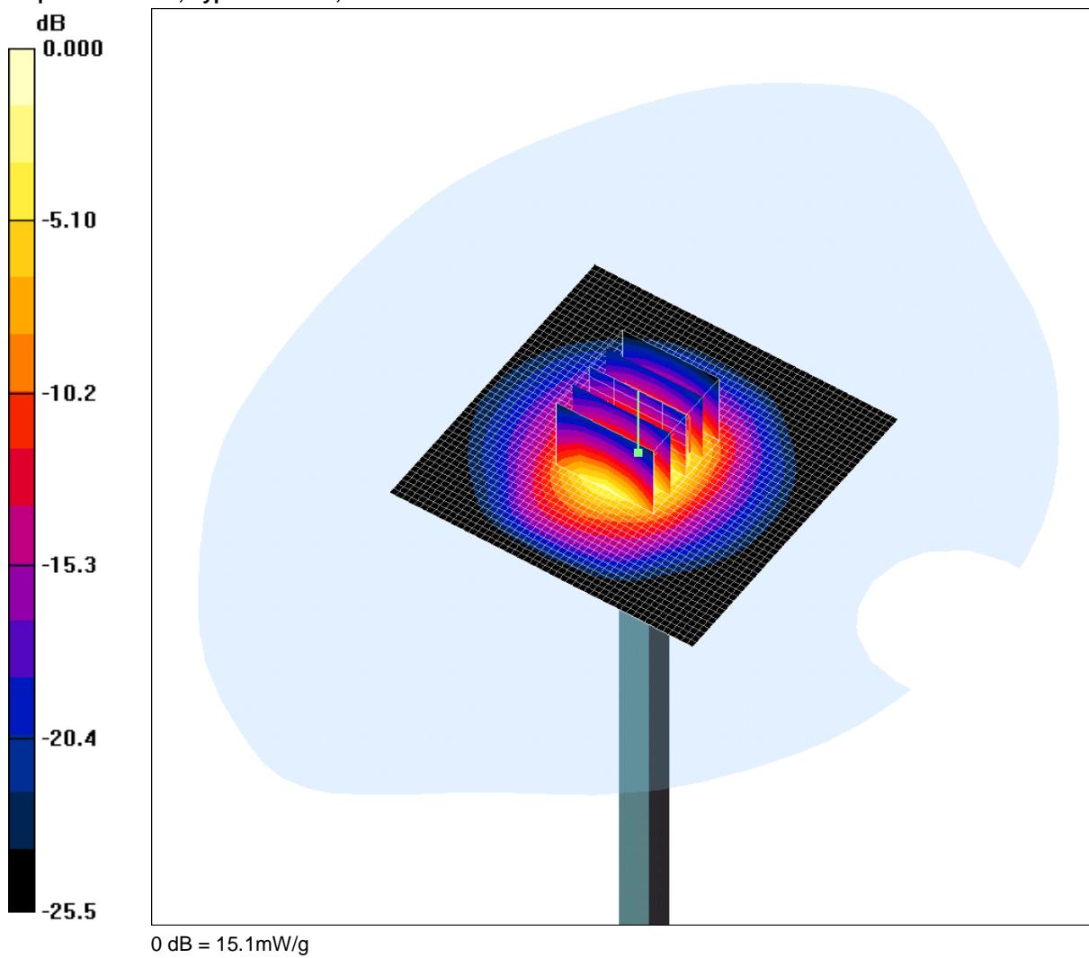
Communication System: CW; Frequency: 2450 MHz; Duty Cycle: 1:1
