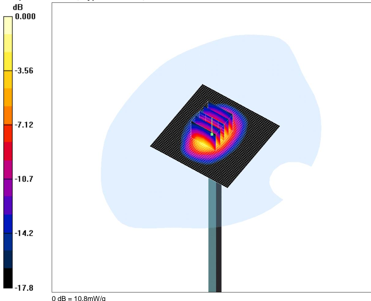
Communication System: CW; Frequency: 1900 MHz; Duty Cycle: 1:1
