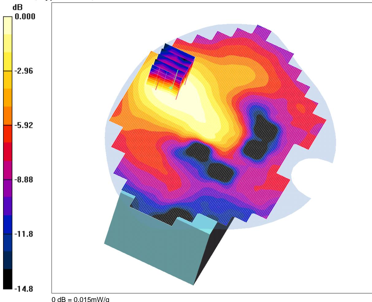
Communication System: PCS 1900; Frequency: 1879.8 MHz; Duty Cycle: 1:8.3
