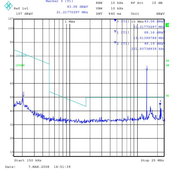
The carrier is shown on the above plot at 13.513MHz
