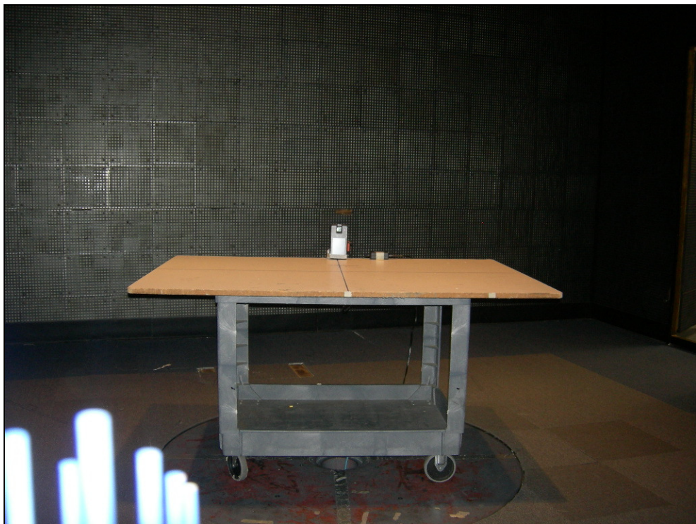
Figure 8: Test Setup – Radiated Emissions Y Position
