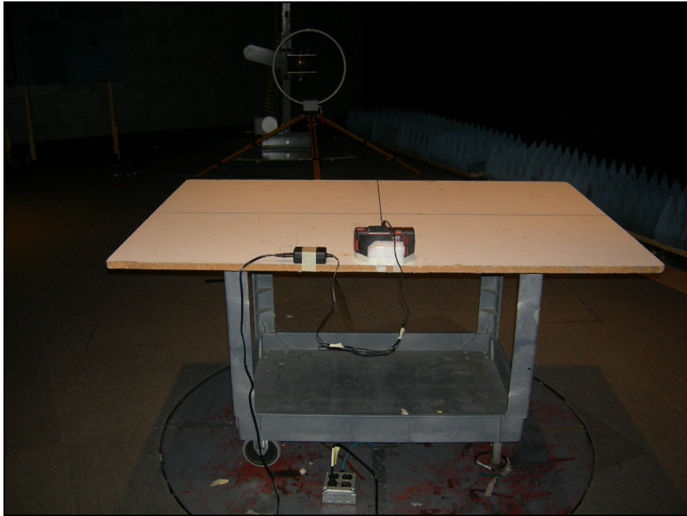
Figure 11: Test Setup – Radiated Emissions Z Position
