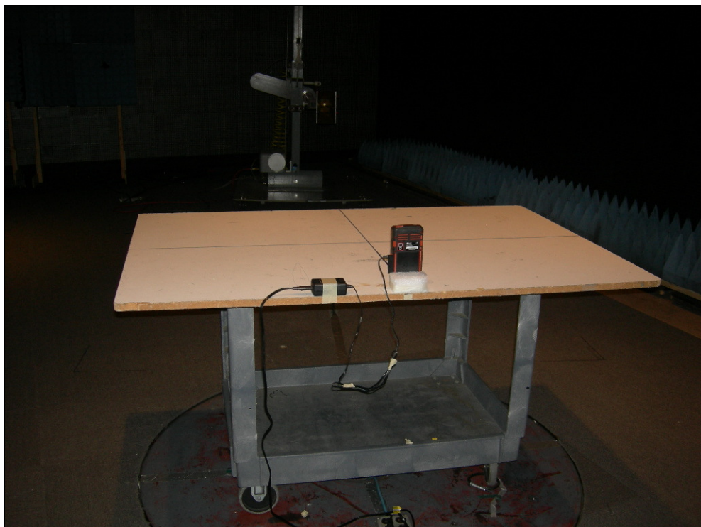
Figure 6: Test Setup – Radiated Emissions Y Position
