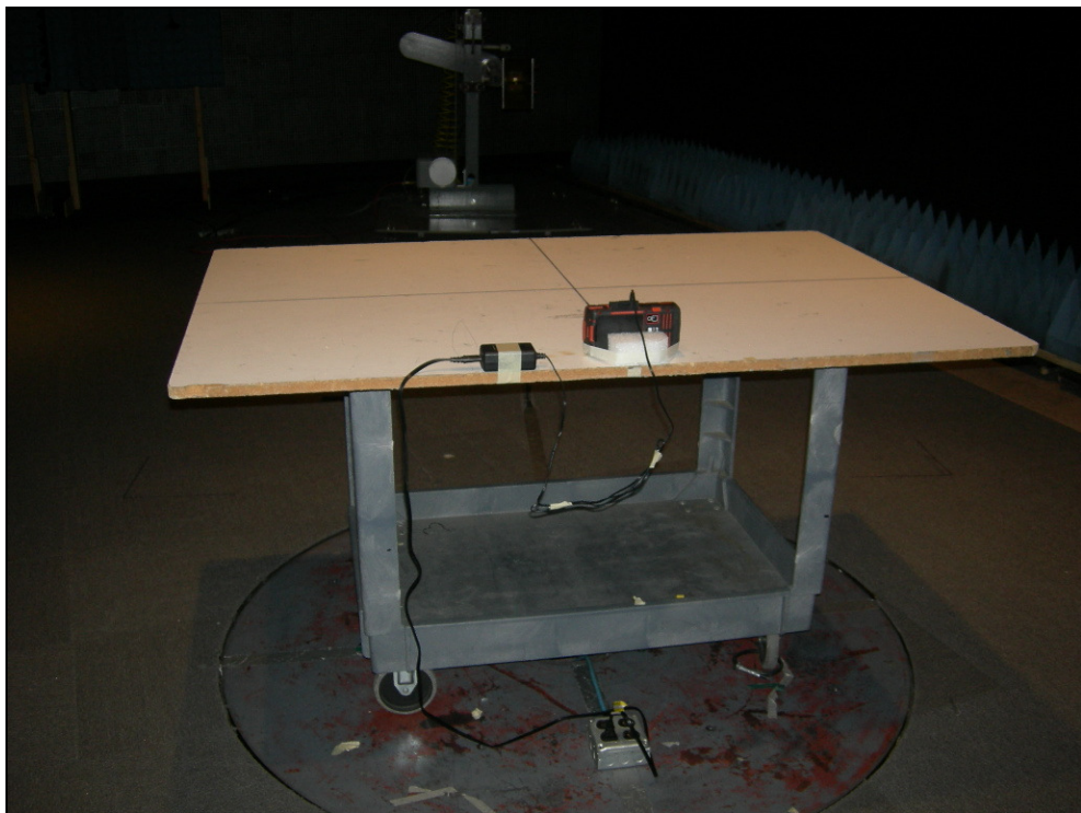
Figure 10: Test Setup – Radiated Emissions Z Position
