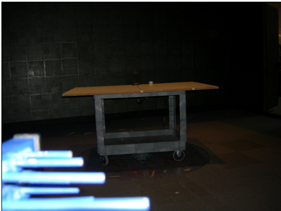
Figure 4: Test Setup – Radiated Emissions X Position
