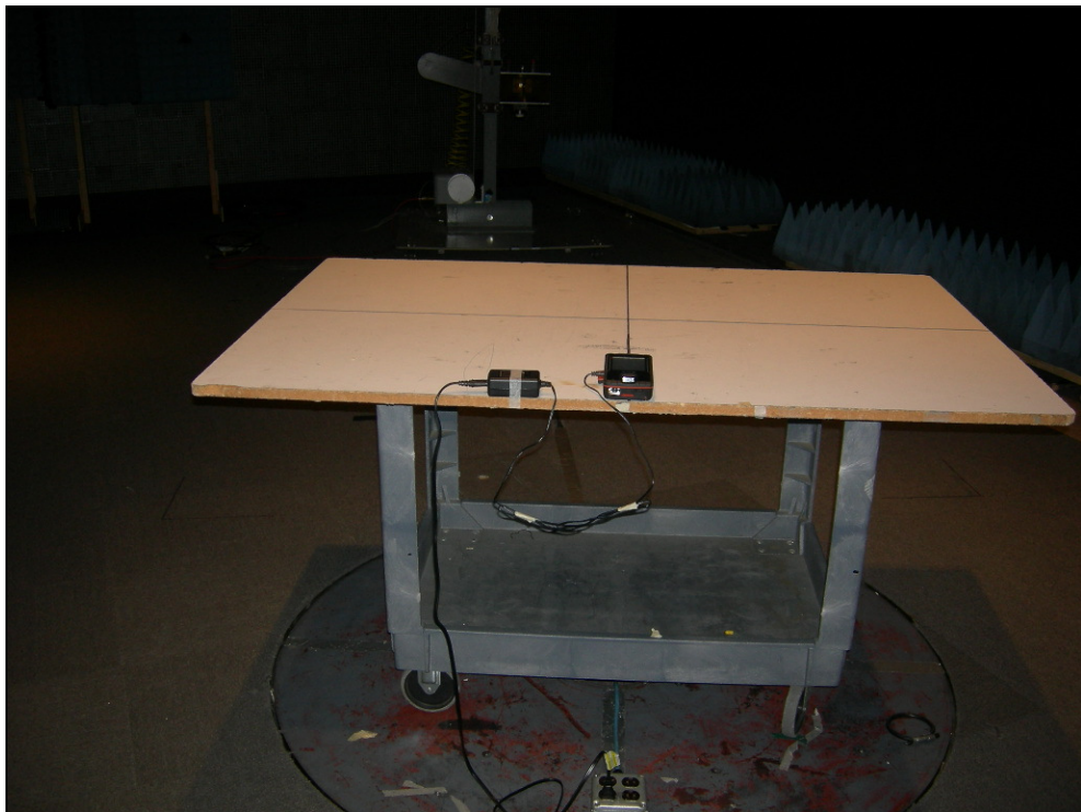
Figure 2: Test Setup – Radiated Emissions X Position
