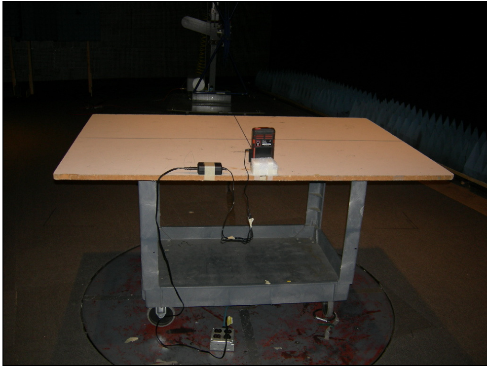
Figure 7: Test Setup – Radiated Emissions Y Position
