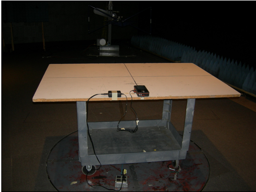
Figure 3: Test Setup – Radiated Emissions X Position
