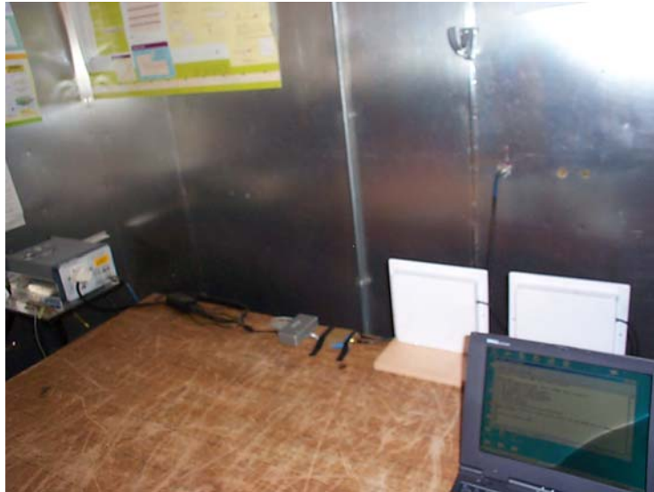
PHOTOGRAPH No. 3 TEST SETUP PLATE ANTENNAS, POWERLINE CONDUCTION
