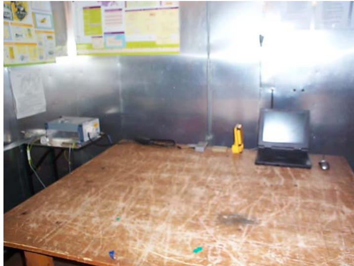
PHOTOGRAPH No. 4 TEST SETUP HANDHELD ANTENNA, POWERLINE CONDUCTION
