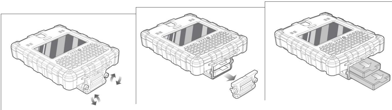
**STEP 1:** loosen Battery cover screws by turning screws anti-clock-wise
