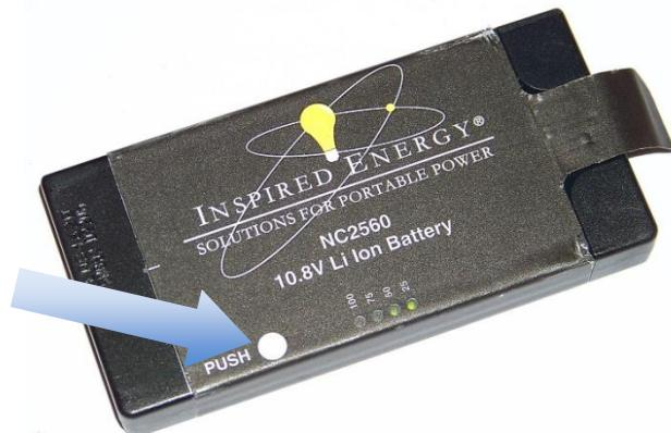
The battery capacity is displayed as the relative State-Of-Charge. Each LED segment represents 25 percent of the full charge capacity. The LED pattern definition is given in the table below. If the battery voltage is below 2.4V/parallel-cell-group, there will be no LED indication.
