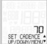
SET CADENCE--LOW LIMIT appears on the display. Press ALTI **A** to reduce the value or **P** to increase it. Once you have set the correct value, press **M** to confirm your setting.
