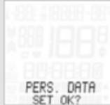
PERS. DATA--SET OK? query. Press **M** in confirmation or **C** to make a correction. The MC 2.0 confirms by displaying PERS. DATA-SET DONE.
