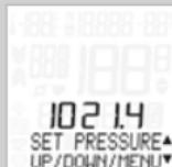
AIR PRESSURE--SET PRESSURE appears on the display. The air pressure number flashes. Press ALTI **A** to reduce the value or **P** to increase it. Once you have set the correct value, press **M** to confirm your setting.
