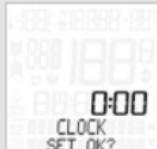
CLOCK--SET OK? query. Press **M** in confirmation. The MC 2.0 confirms by displaying CLOCK--SET DONE.
