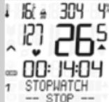
**STOPWATCH:** independent stopwatch for measuring times/intervals.
