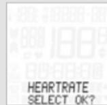
CADENCE or HEARTRATE or NONE--SELECT OK? is shown in display. Press **M** in confirmation.
