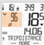
After pairing the cadence transmitter, the current cadence is shown in area 2 of the display. In function mode, the cadence information can be accessed by pressing the button P/CAD
