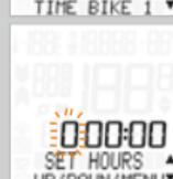
TIME BIKE 1-SET HOURS appears on the display. The hours flash. Press ALTI **A** to reduce the value or **P** to increase it. Once you have set the correct value, press **M** to confirm your setting.
