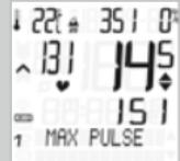
**MAX PULSE:** shows the maximum (highest) heart rate for the current trip (since the last reset).
