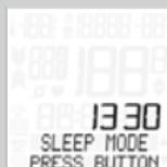
The MC 2.0 goes into sleep mode after five minutes if no speed signals are received. SLEEP MODE--PRESS BUTTON appears on the display.
