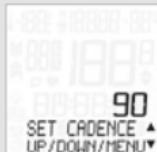
SET CADENCE--HIGH LIMIT appears on the display. Press ALTI **A** to reduce the value or **P** to increase it. Once you have set the correct value, press **M** to confirm your setting.
