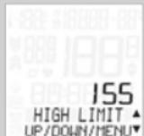
SET PULSE--HIGH LIMIT appears on the display. Press ALTI **A** to reduce the value or **P** to increase it. Once you have set the correct value, press **M** to confirm your setting.
