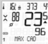
**MAX CAD:** shows the maximum cadence of the current trip (since the last reset).
