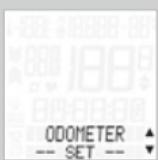
Press **P** to scroll to ODOMETER---SET---. Press **M** in confirmation.
