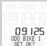
ODO BIKE 1 (or BIKE 2)---SET OK? Press **M** to confirm or **C** to make a correction.
