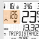
After pairing the PULSE transmitter, the current heartrate is shown in area 2 of the current HR display. In function mode, the functions can be accessed by pressing the button P/CAD **P**. RESETTING the trip data also resets the HR data to zero.
