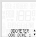
ODOMETER ODO BIKE 1 or ODO BIKE 2 is shown on the display. Press ALTI **A** or **P** to make a selection. Press **M** in confirmation.
