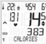
**CALORIES:** shows the calories burnt on the current trip (since the last reset).
