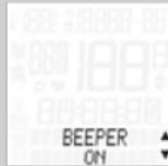
BEEPER--ON or OFF appears on the display. Press ALTI **A** or **P** to make a selection. Press **M** in confirmation. BEEPER ON (or OFF)--SET OK? Press **M** in confirmation.
