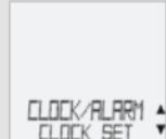
Using **▲▼** go to CLOCK/ALARM/SET. Confirm with **M**.
