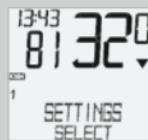
Using **▲▼** go to SETTINGS/SELECT. Confirm with **M**. You are now in setting mode (pressing **C** for 3 seconds gets you back to function mode).
