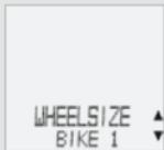
WHEELSIZE/BIKE 1 (use **▲▼** to go to setting for bike 2). Confirm with **M**.
