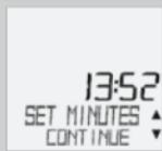
CLOCK...SET MINUTES/CONTINUE. Set the minutes using **▲▼**. Confirm the minutes setting with **M**.
