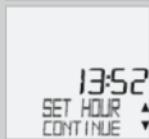
CLOCK...SET HOUR/CONTINUE. Set the hours using **▲▼**. Confirm the hour setting with **M**.
