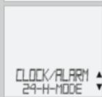
CLOCK/ALARM/24-H-MODE. You can switch to 12-H mode using **▲▼**. Confirm with **M**.
