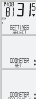
Using ▲▼ go to SETTINGS/SELECT. Confirm with M. You are now in setting mode (pressing C for 3 seconds gets you back to function mode).
