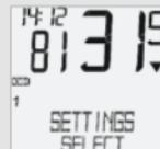
Using go to SETTINGS/SELECT. Confirm with . You are now in setting mode (pressing for 3 seconds gets you back to function mode).
