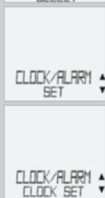
Using **▲▼** go to CLOCK/ALARM/SET. Confirm with **M**.
