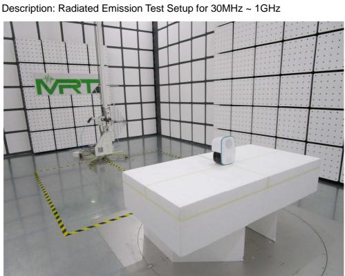
Test Mode: Mode 1~2 Description: Radiated Emission Test Setup for 30MHz ~ 1GHz
