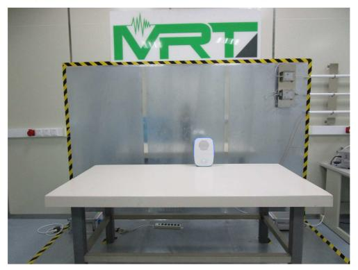
Test Mode 1~2 Description: Back View of Conducted Emission Test Setup
