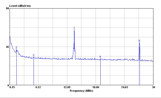
No signal can be detected from 9kHz to 150kHz, so the graphs are omitted below 150kHz.
