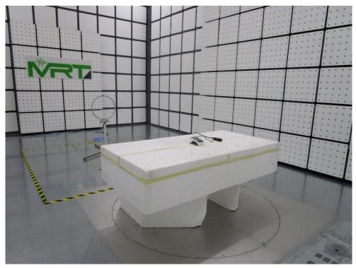
Test Mode: Mode 1 Description: Radiated Emission Test Setup for 30MHz ~ 1GHz
