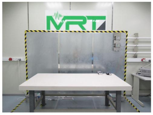
Test Mode: Mode 1 (Adapter: PA150-090T1A500) Description: Back View of Conducted Emission Test Setup
