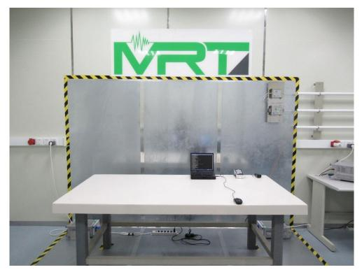
Test Mode: Mode 3 (Adapter: BA048-090500MAX) Description: Back View of Conducted Emission Test Setup
