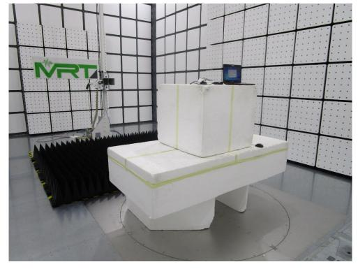
Test Mode: Mode 1/Mode 2 Description: Conducted Emission Test Setup
