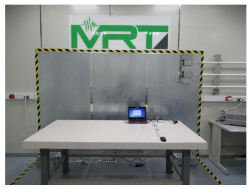
Test Mode: Mode 1 (Adapter: BA048-090500MAX) Description: Back View of Conducted Emission Test Setup
