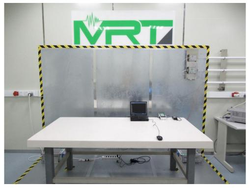
Test Mode: Mode 3 (Adapter: PA150-090T1A500) Description: Back View of Conducted Emission Test Setup
