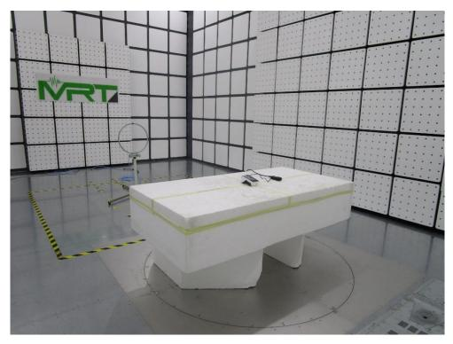
Test Mode: Mode 1 (Adapter: BA048-090500MAX) Description: Radiated Emission Test Setup for 30MHz ~ 1GHz
