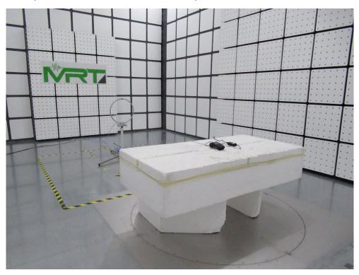
Test Mode: Mode 1 Description: Radiated Emission Test Setup for 30MHz ~ 1GHz
