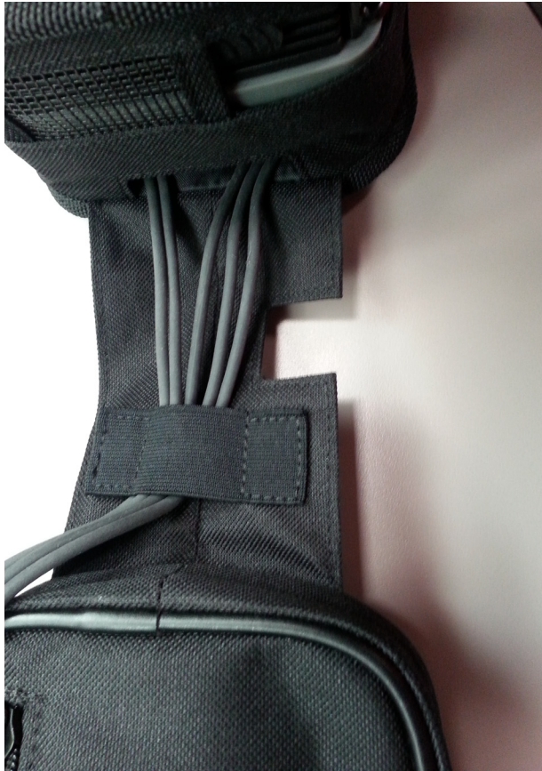
Figure 15 Cable routing through the hinge of the glove
