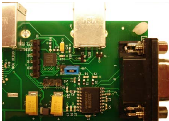
Figure 3-5. Jumper Set For RS-232 Serial Communications
