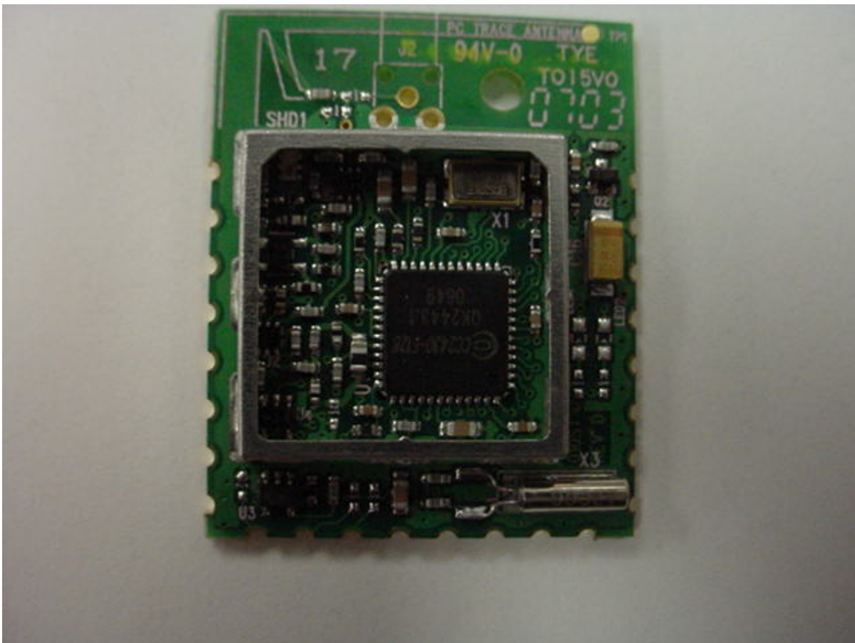
Photo One B – Internal Open for Inspection – Shield Removed
