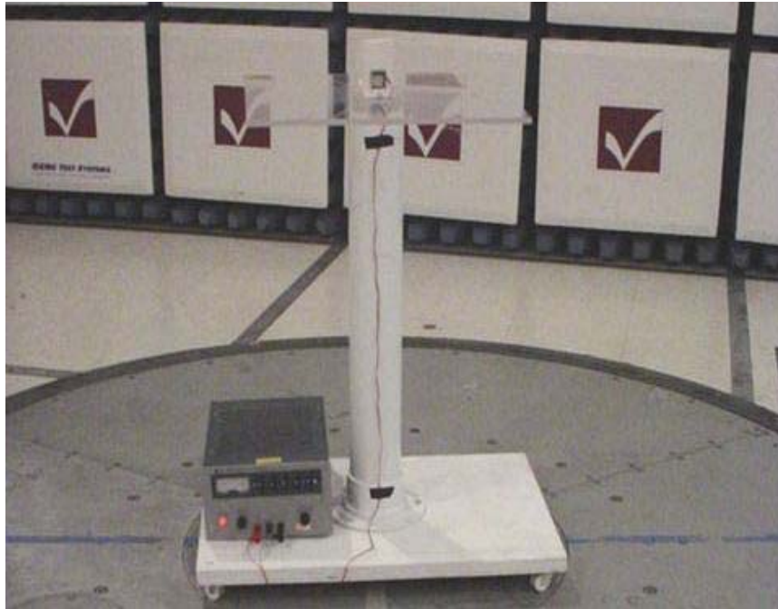
Horizontal Orientation, EUT on Test Pedestal, F antenna
