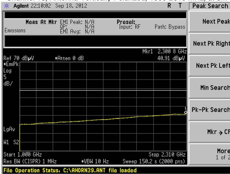
Channel 18, Antenna Vertically Polarized, 1000-2310 MHz, at 3m
