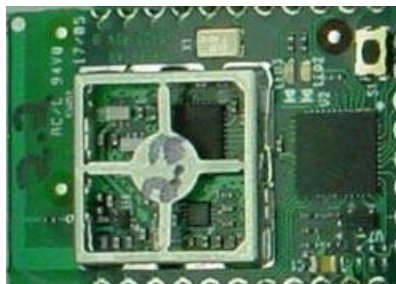
Figure 2-1. Top-Side of RF FreeStar Module
