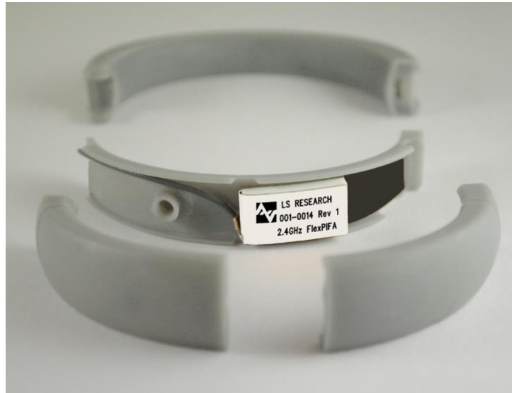
Figure 30 FlexPIFA Integrated into Bracelet
