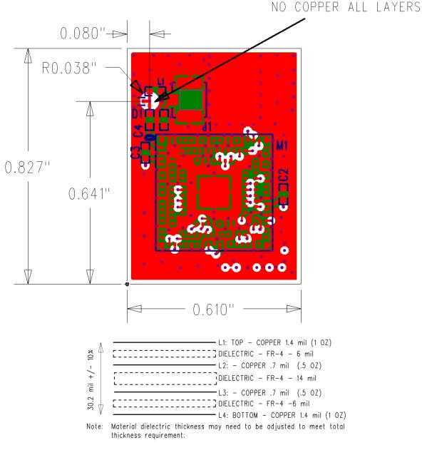
Figure 4 SIP Module with U.FL (External Antenna) Reference Design
