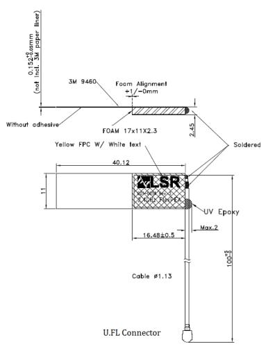
Figure 9 LSR 2.4 GHz FlexPIFA Antenna Dimensions
