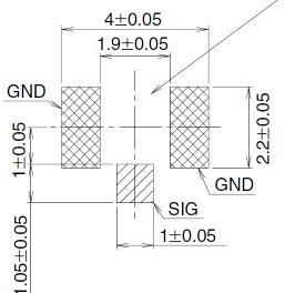
Figure 6 U.FL Connector Drawing
