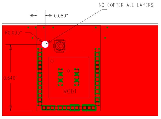
Figure 5 Host PCB for Sterling-LWB U.FL Module Variant
