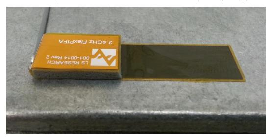
Figure 27 FlexPIFA Mounted on Metal
