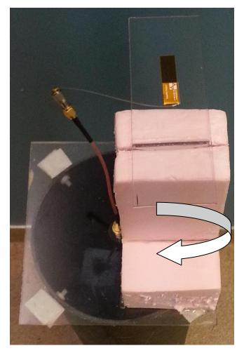
Figure 19 Flat Orientation Set-Up
