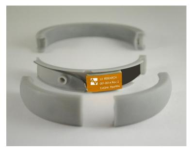
Figure 30 FlexPIFA Integrated into Bracelet
