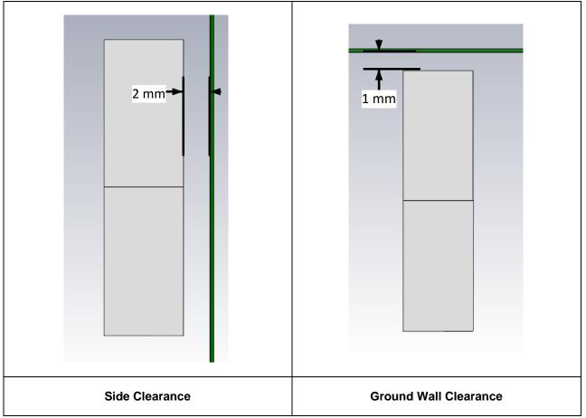
Figure 23 Side and Ground Wall Clearance
