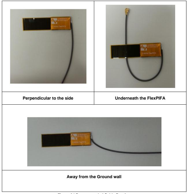
Figure 24 Recommended Cable Routing
