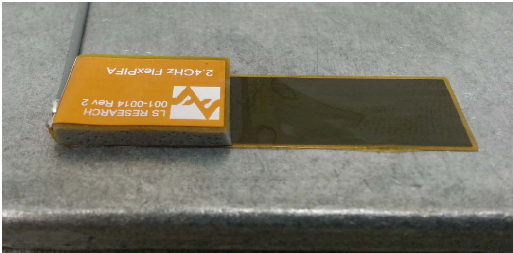
Figure 27 FlexPIFA Mounted on Metal
