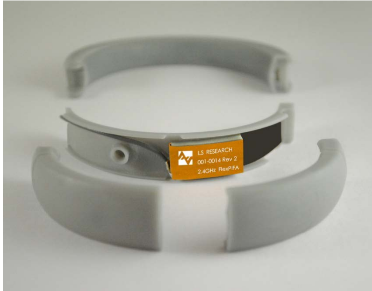
Figure 30 FlexPIFA Integrated into Bracelet
