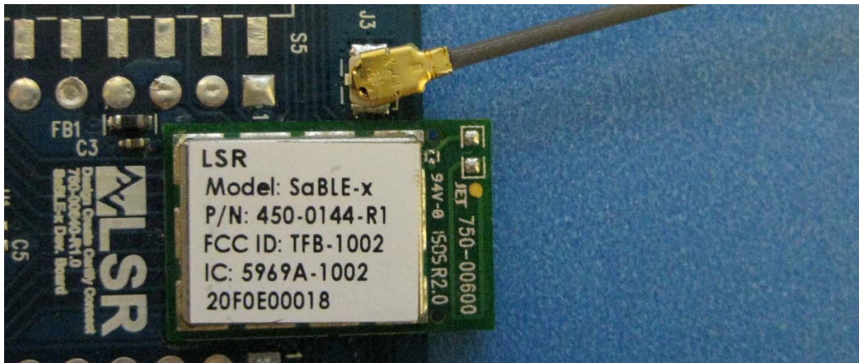
u.fl cable connection (Picture 2)
