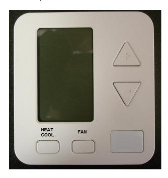
There are 4 buttons on the unit, namely HEAT COOL, FAN, Up Arrow and Down Arrow. The following are the functions of these buttons. **HEAT COOL** – To select OFF, HEAT or COOL mode. **FAN** – To change the fan speed to HIGH speed or LOW speed setting or OFF. **UP Arrow/DOWN Arrow** – To increase (Up) or decrease (Down) temperature setting.
