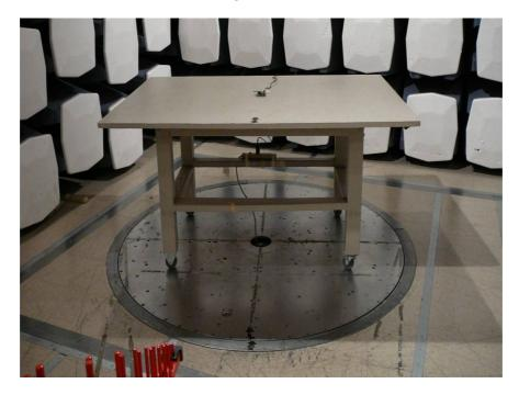
14.5 Radiated Emissions below 1 GHz (Integral Antenna) – Front View
