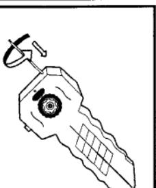
Tighten the antenna into the transmitter.
