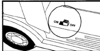
The power switch is located by the side of the vehicle (as shown). Please make sure it is the ON position when you operate, and OFF position when not in use.
