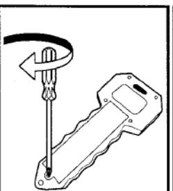
Unscrew battery cover with a screwdriver (not included).
