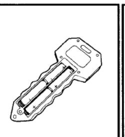
Install four (4) AA batteries (not included) with polarity (+/-) as shown inside battery compartment.
