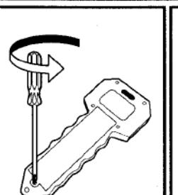
Close battery cover and tighten screw.
