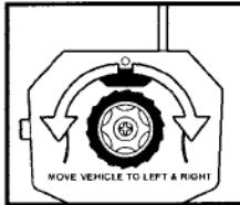
To move the vehicle to the left, turn the navigation button anti-clockwise. To move the vehicle to the right, turn the navigation button clock-wise.
