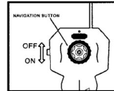
The power switch is located by the side of the transmitter (as shown). Please make sure it is the ON position when you operate, and OFF position when not in use.
