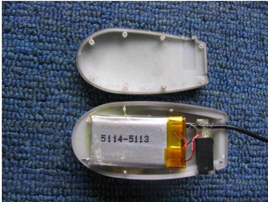
EUT Battery and Housing View
