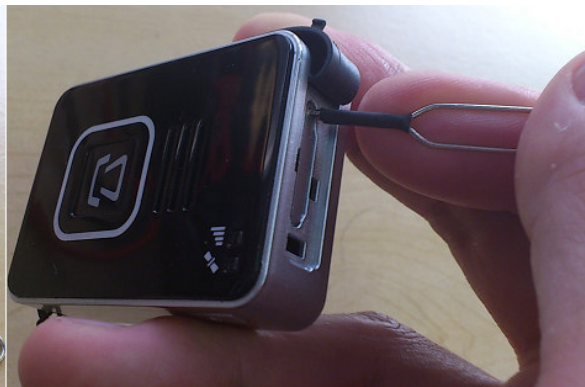
B. Insert the pin into the small hole
