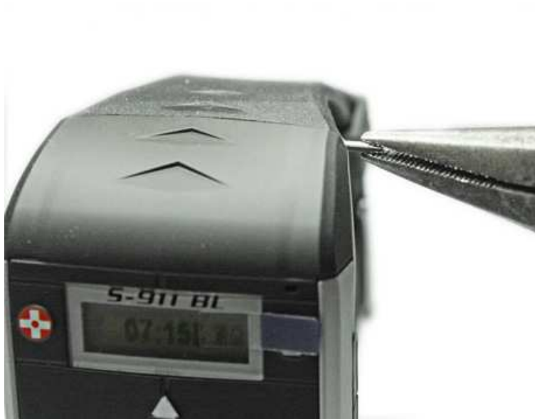
Fig 5. Pull out the 2 pins with long nose pliers
