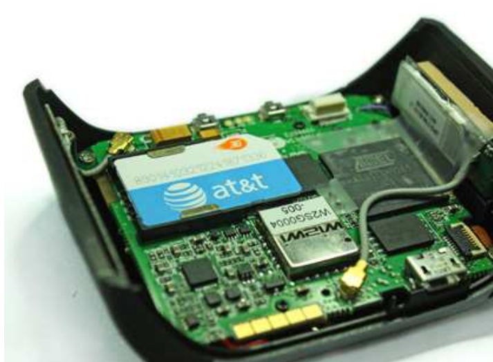
Fig 8. Fully insert SIM card into the card holder
