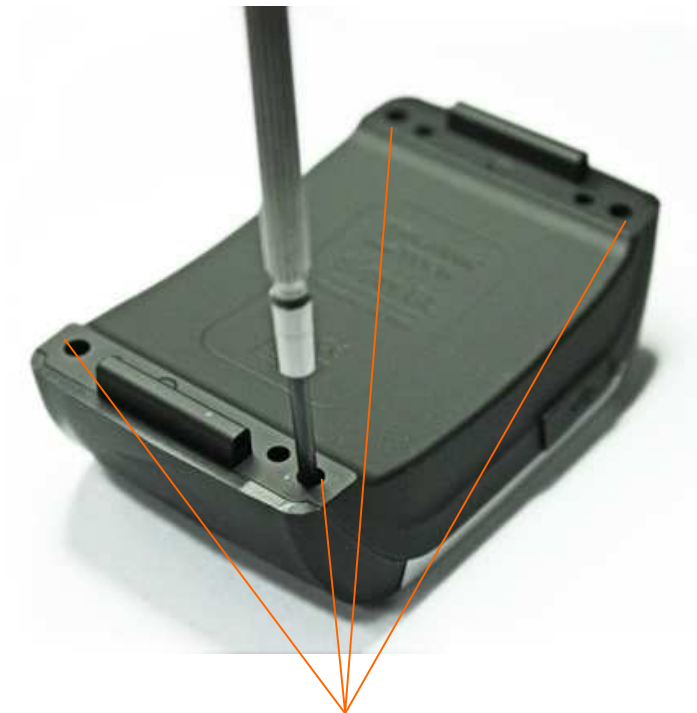
Fig 6. Unscrew the 4 rear case screws
