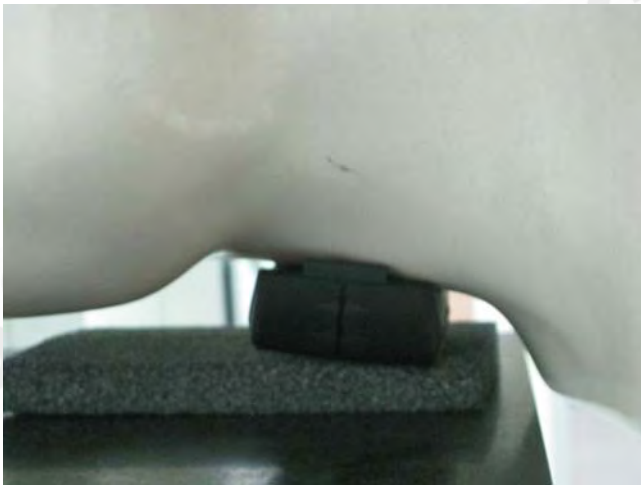
Fig.4 EUT back side touch to the neck part of SAM phantom with headset.
