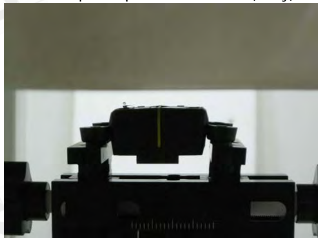
Fig.3 EUT front side touch to the flat phantom (1.0 cm gap between the front side of EUT and flat phantom)
