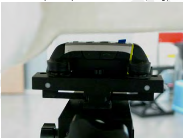
Fig.3 EUT front side touch to the flat phantom (1.0 cm gap between the front side of EUT and flat phantom)
