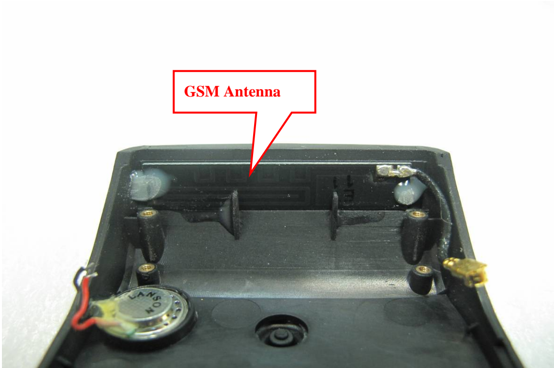
Internal View of EUT – 7 (GSM Antenna)
