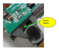
The Power Button is the only operation button on the device. When Lola HT 2 is under "Normal Mode", the power button is used for powering on and off the device.
