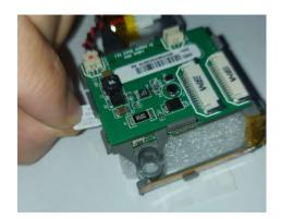
Insert a Nano-SIM, and push the Nano-SIM to the end, and it will be locked. See the orientation of the Nano-SIM before inserting the SIM.
