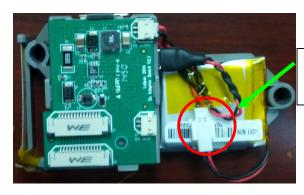
2 pin connector is used to connect the battery and the main board
