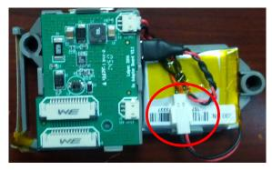
• Remove the connection between the DC/DC adaptor board and the mainboard
