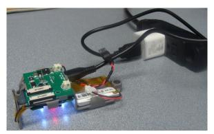
• Wait for 20 seconds, press the power button for more than 3 seconds to turn off the Lola HT 2. This step ensures that the device is generating a reset when it is connected to the utility software.
