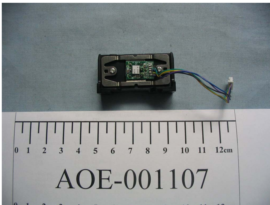
FIGURE 22 WIRELESS POINT OF SALE PDA (M/N: MRT320) HAND-HELD UNIT CARD READER MODULE (SIDE 2)
