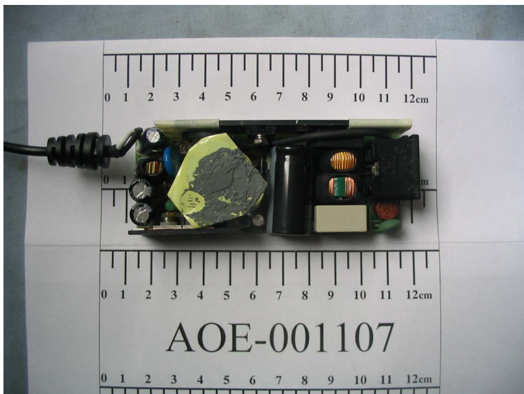
FIGURE 39 WIRELESS POINT OF SALE PDA (M/N: MRT320) AC ADAPTOR MAIN BOARD (COMPONENT VIEW)
