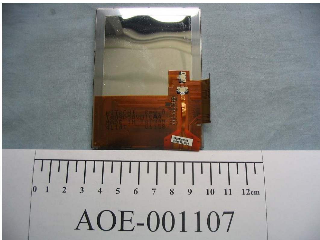
FIGURE 19 WIRELESS POINT OF SALE PDA (M/N: MRT320) HAND-HELD UNIT LCD PANEL (SIDE 1)
