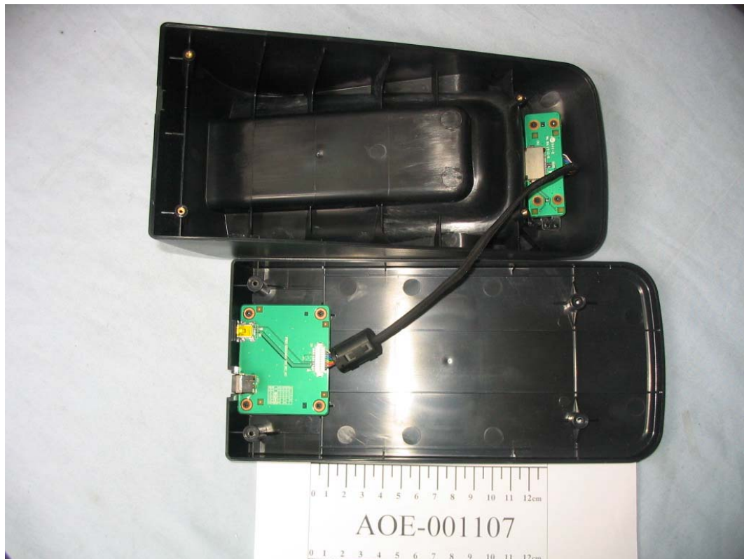
FIGURE 30 WIRELESS POINT OF SALE PDA (M/N: MRT320) CHARGING CRADLE (COVER REMOVED)
