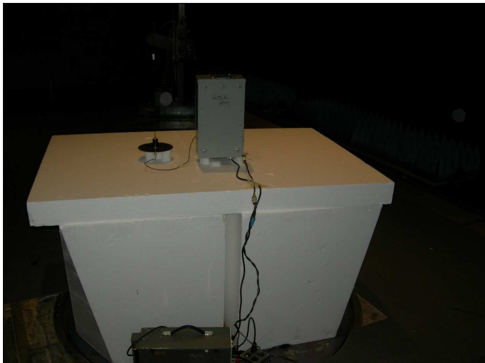
Figure 4: Radiated Emissions – S4x Meter Host
