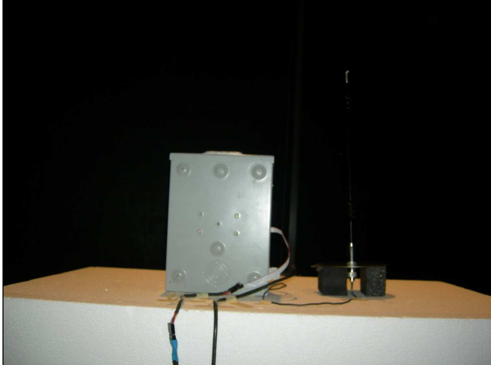
Figure 2: Radiated Emissions – Focus AX Meter Host
