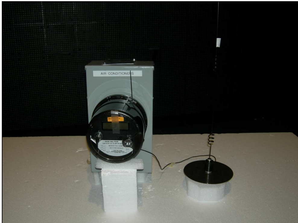
Figure 3: Radiated Emissions – S4x Meter Host
