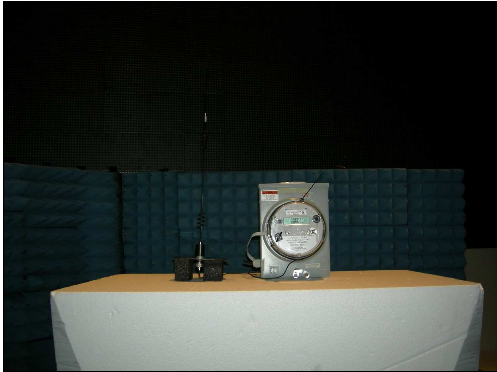
Figure 1: Radiated Emissions – Focus AX Meter Host
