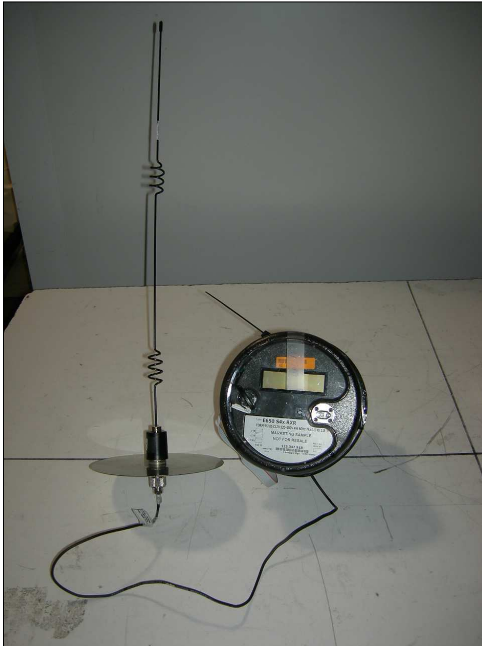
Figure 2: External Photo – S4x Meter Host
