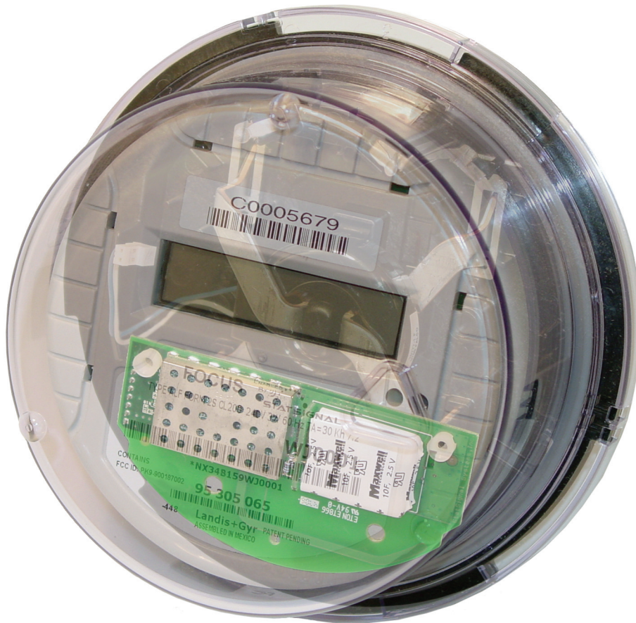
Figure 1. The Hunt Technologies StatSignal FOCUS Endpoint Module and L+G FOCUS Meter
