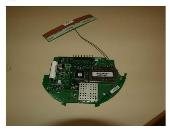
Front with Shields with shields removed.
