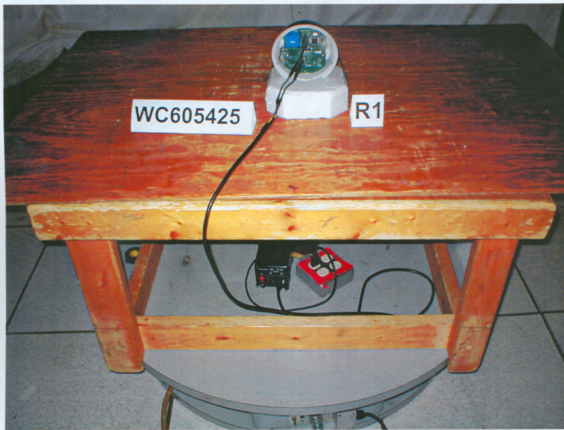
Figure 2: Rear View of Radiated Emissions Setup
