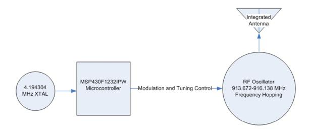
This device is an RF transmitter to be used with Itron's system. It transmits On-Off-Keyed signals to compatible Itron receivers. It has a digitally-tuned Voltage Controlled Oscillator. It's transmit frequency is random and covers a 2.5 MHz band nominally. At room temperature, the transmitter is digitally tuned (i.e. minimum and maximum values are stored in EEPROM memory) so that its minimum transmit frequency is 913.672 MHz and its maximum transmit frequency is 916.138 MHz.
