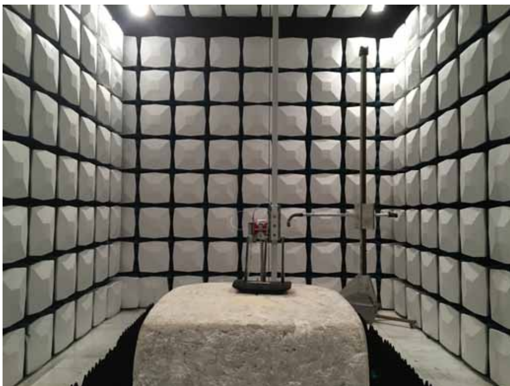
Description: Radiated Emission Test Setup for 1~18GHz
